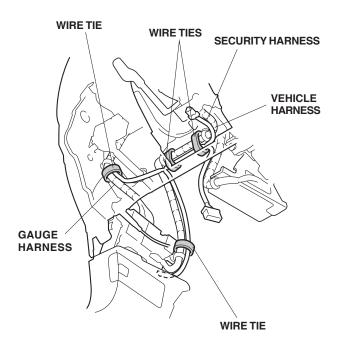
20. Position the upper steering column cover above the steering column, and plug the security harness 2-pin connector into the LED 2-pin connector.
