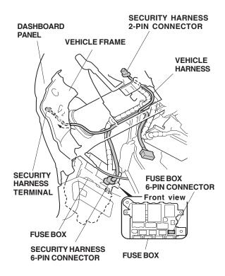
Route the security harness 2-pin connector along the vehicle harness. Route the security harness terminal between the vehicle frame and dashboard panel. 18. Remove the vehicle ground bolt, and attach the security harness ground terminal using this bolt.
